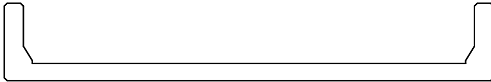
CONCRETE SLAB BRIDGE - TYPE "CSL"
